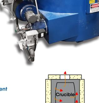
A burner assembly spirals heat around a cast iron pot or crucible to provide maximal efficiency. The exhaust gas exits the system through a side flue or the top cover of the furnace.
